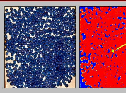
Defect not visible to the human eye, easily seen with hyperspectral classification.
