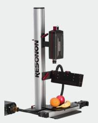
The linear stage holds the sample and translates across the field of view. Used for small samples that are easy to move.
