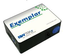
The Exemplar<sup>™</sup> is the next step in the evolution of miniature CCD spectrometers. It is the first smart spectrometer featuring on board data processing, USB 3.0 communication, and temperature compensation. The Exemplar is also optimized for multi-channel operation featuring ultra-low trigger delay, ultra low gate jitter, and super speed data transfer. Additionally, the Exemplar features a 2048 element detector, and built-in 16-bit digitizer with a >2.0 MHz readout speed.
