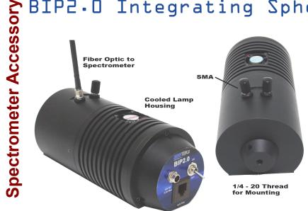
BIP2.0 is a compact, fiber coupled integrating sphere device designed as a sampling accessory for measuring diffuse reflectance using any fiber optic spectrometer from B&W Tek, Inc. The two inch diameter integrating sphere is machined from PTFE which is highly reflective (>97%) over a broad spectral range of 350 to > 2600nm.
