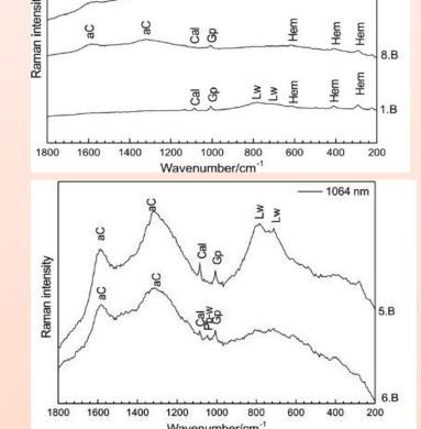
Raman spectra collected in the medallion representing "The Art Painting" by using 1064 - nm line on a: skin color (point reddish layers (points 1.B and 9.B) and grayish layers (points 5.B and 6.B) aC= amorphous carbon, Cal= calcite,
