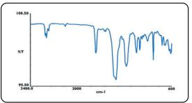
Small polymer pellet measured with a Germanium crystal
