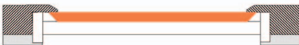
Trough plate HATR crystal plate – ideal for liquids, powders, pastes and gels.
