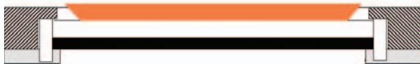
Flat plate HATR crystal plate – ideal for solids, polymer films and coatings.
