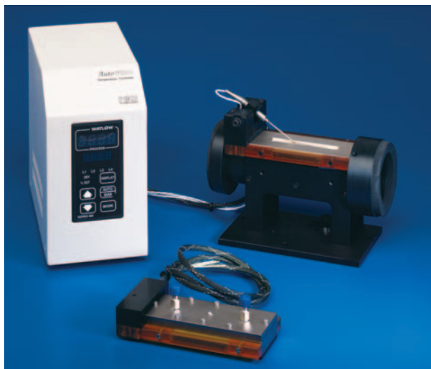
HATR with Heated Trough Plate and Sample Temperature Thermocouple – foreground shows Heated Flow-Through Cell.
