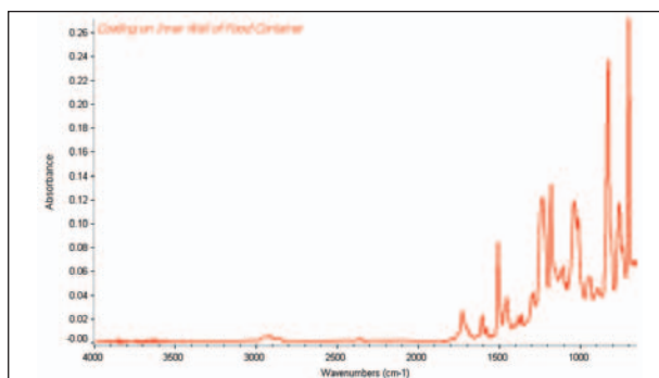
FTIR spectrum of coating on inner wall of food container by HATR with ZnSe flat plate and pressure plate.
